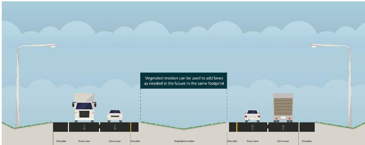
Figure 9. At-Grade Highway Cross Section (Six Lanes)
