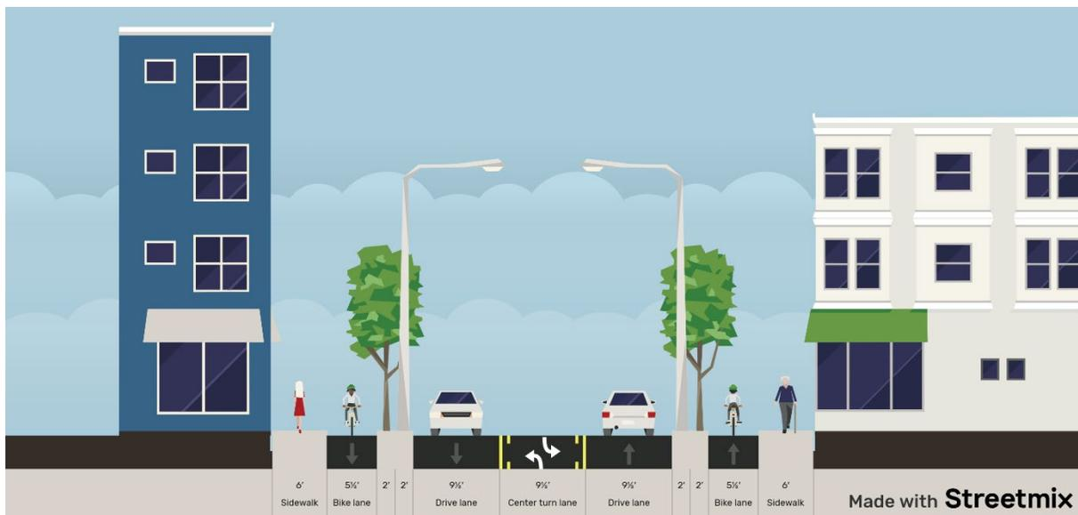
Figure 13 shows a concept for a potential Ingra Street that fits within the existing 60-foot-wide right-of-way. It features a shared directional cycle track/sidewalk (see Figure 14) on each side and includes a center turn lane to access driveways or side streets. A 4-foot buffer would separate the vehicle travel lanes from the nonmotorized facilities.
