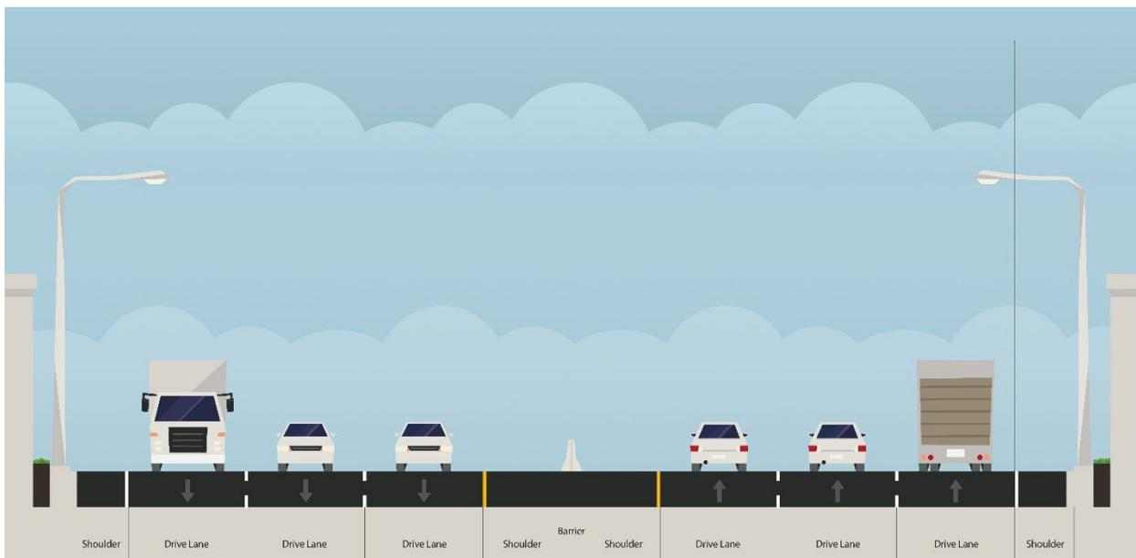
Figure 8. At-Grade Highway Cross Section (Four Lanes)
